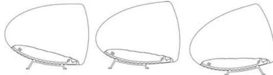
Figure 2 Using the centre speaker foot to adjust the angle
